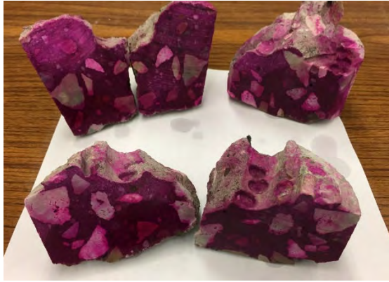
Fig. 13. Cuyahoga carbonation depth results -S&T
