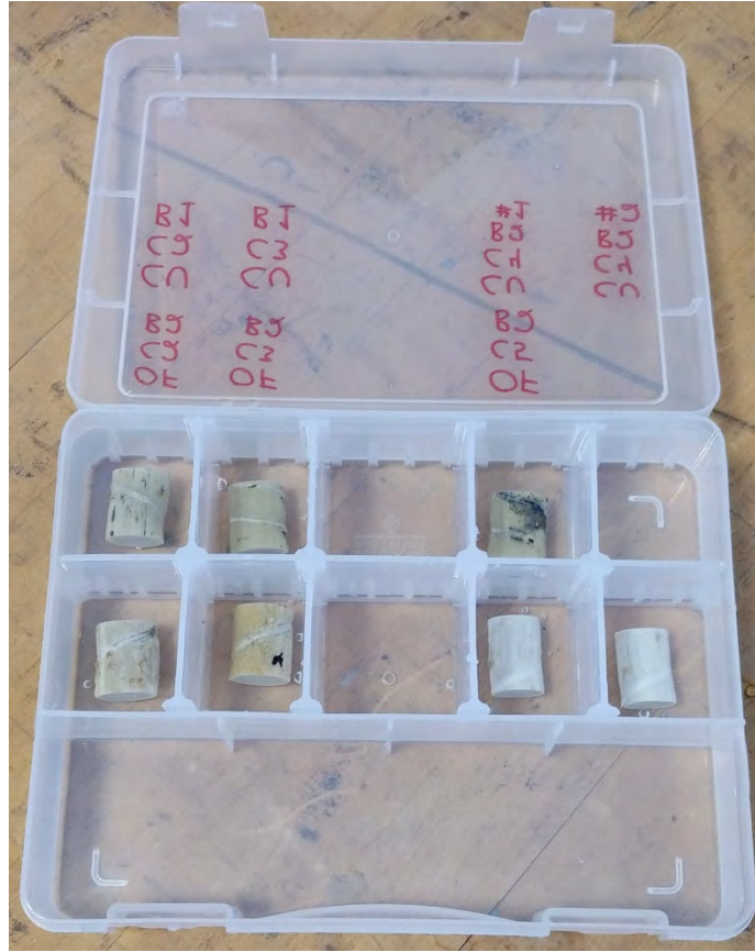
Fig. 37–Moisture uptake specimens immersed in distilled water
