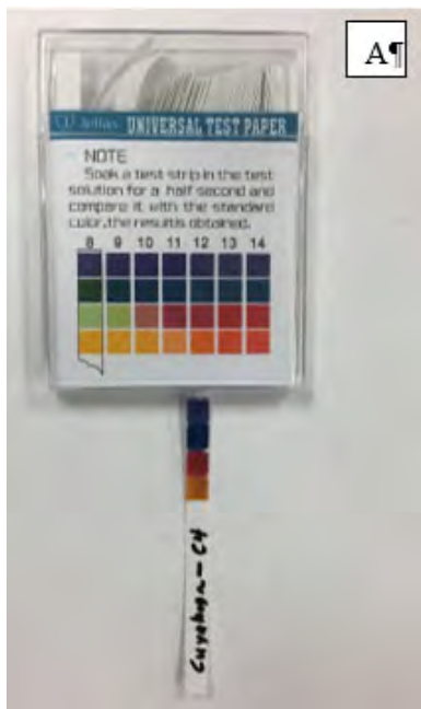
Fig. 60—pH color range for Cuyahoga core 4
