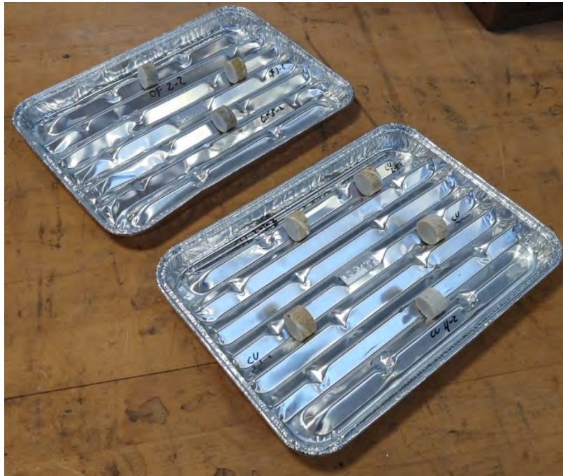
Fig. 40–Dry-out specimens in corrugated aluminum pans
