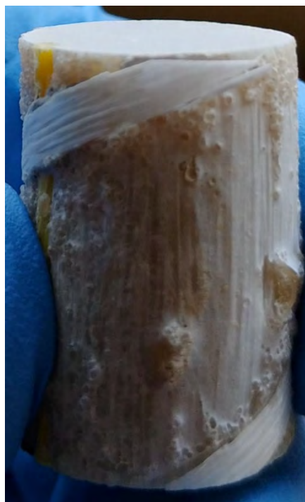
Fig. 8. Part of the helical wrap fell off of OH2_C4_B2-2
