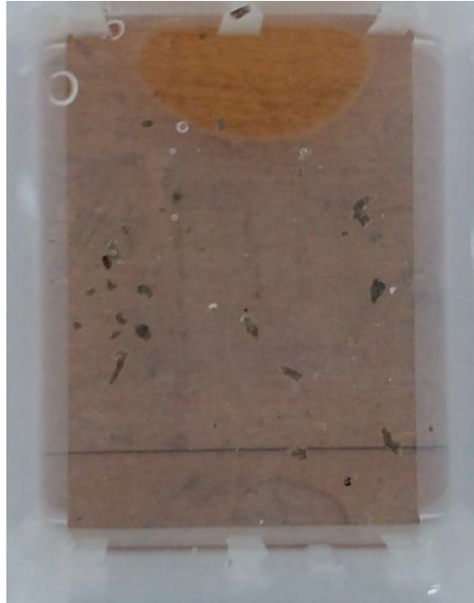
Fig. 6. Sand particles at the bottom of the immersion chamber of CO_C5_B2
