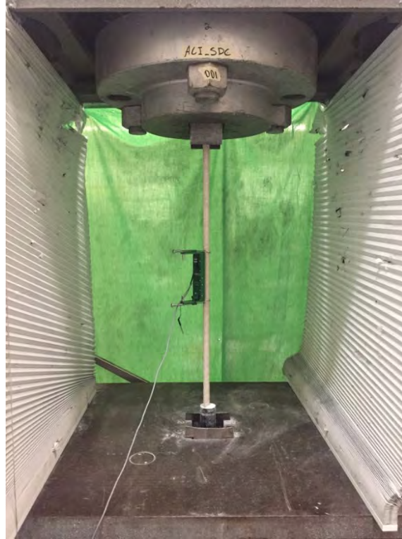
Fig. 51. Full size virgin bar test set up
