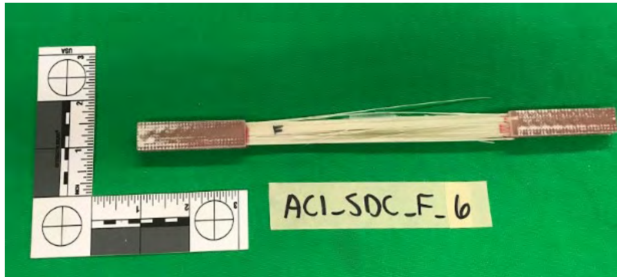
Fig. 41. Coupon F_6 after failure
