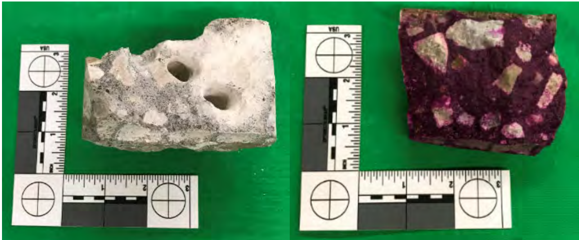
Fig. 59–Cuyahoga Core 4 pH test with phenolphthalein
