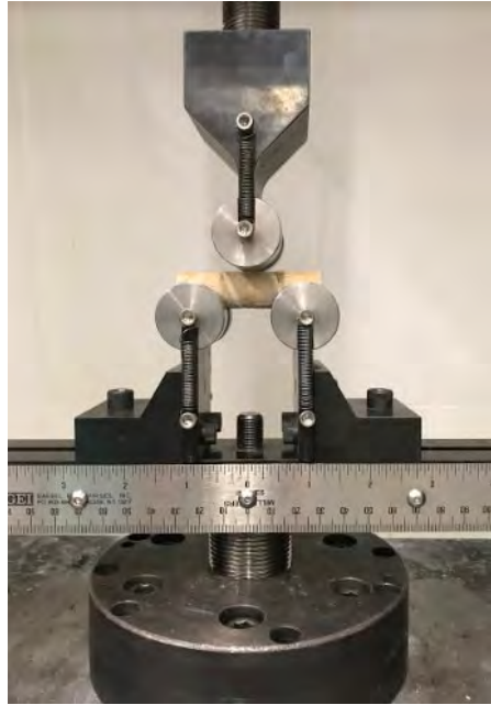
Fig. 39–Horizontal shear test setup
