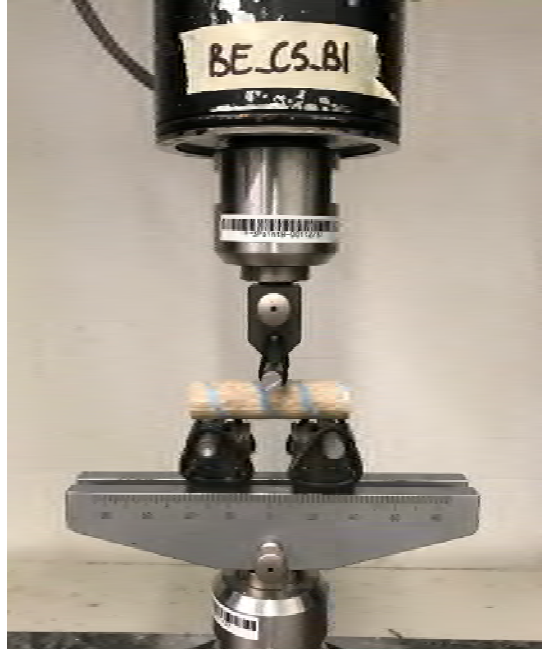
Fig. 47–Modified horizontal shear test setup for short bars
