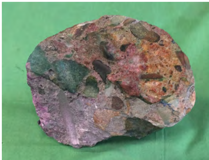
Fig. 61—McKinleyville pH range using the rainbow indicator
